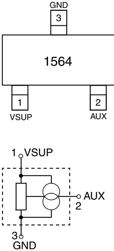
**Fig. 4–5:** Pin configuration
