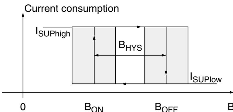
**Fig. 4–9:** Definition of magnetic switching points for the HAL 1564
