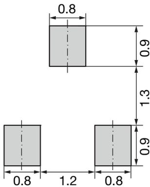
**Fig. 4–3:** SOT23 footprint for reflow soldering
